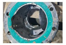
**CHALLENGE**: Typical valves show extreme solids buildup or accelerated erosion after only a few months of service in harsh pulp & paper applications.
