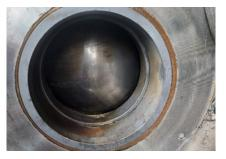
**SOLUTION**: Bray's S19L valves show no signs of abrasion or erosion after 24+ months of service in similar severe service applications.
